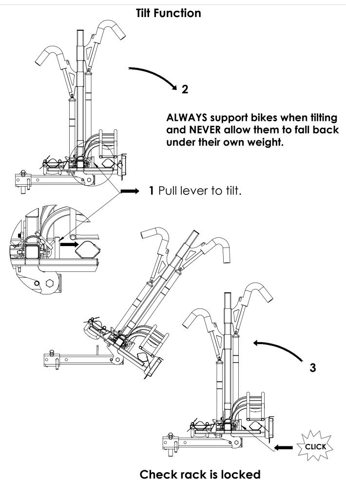
Check rack is locked in upright position before driving.
