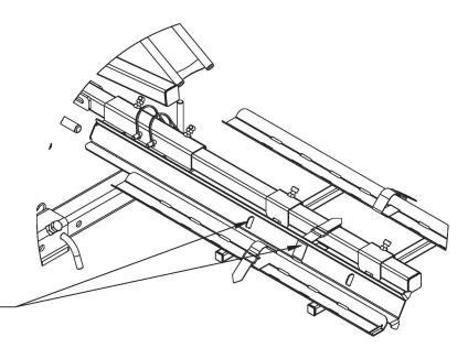
Stow Ramp on Carrier & secure with Cinch Strap when travelling. —
