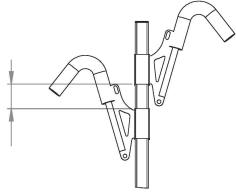
NOTE: There must be a gap between the Hooks. Adjust bike position if necessary.
