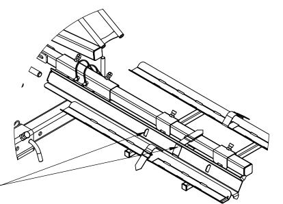
Stow ramp on carrier & secure with cinch strap when travelling.
