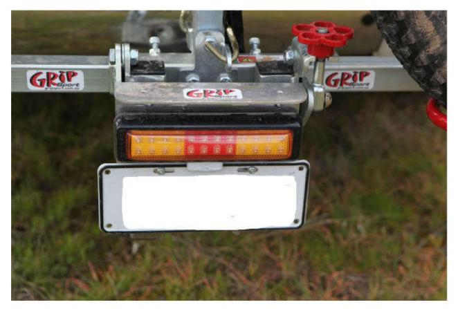
The optional LED number plate mount is a handy addition. Loosening the red knob on the right allows the rack to tilt.
