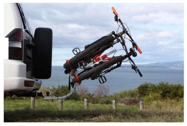
The tilting action is super easy but really designed for horizontally split doors and hatches it didn't provide much clearance for the barn door on my vehicle.
